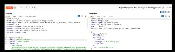
Figure 17: Reflected unsanitized input on API response in id parameter
